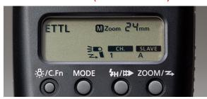
When the 430EXII is set to this option it will function as a remote slave flash unit controlled by a master flash unit such as a Canon 580EX II or ST-E2 Speedlite Transmitter. The master and slave(s) must be set to the same communication channel. Slaves set to a different channel than the master will not trigger. You can select from four channels, numbered 1-4.
